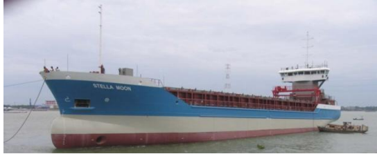
STELLA MOON, produced for Stella Shipping, Denmark By Ananda shipyard. 2900 dwt MULTIPURPOSE CARGO VESSEL
